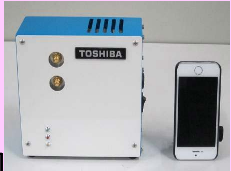
2L size receiver unit at 77 K cooled by Starling cycle cryogenic system.
