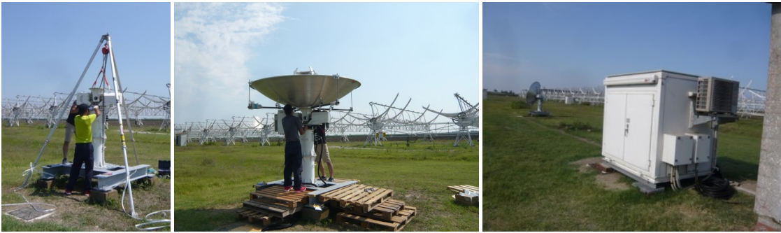
Fig. 2 Installation of transportable VLBI station at Medicina. The transportable 2.4m antenna consists of separate assemblies for the dish and Az/EI drive system. Three persons are sufficient to assemble the system in two days of work (Left and Center). A small air-conditioned box, located 30 m from the antenna, contains antenna control system(right).
