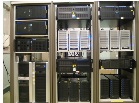
Fig. 1 Cluster computer of correlators system by using GICO3 Software correlator at NICT/Kashima.
