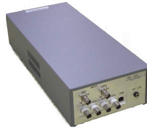
Fig. 3 One unit of K5/VSSP32 sampler has four video signal inputs. Data output and remote control is made via USB2.0 interface. One geodetic terminal of 16 video signals is composed of four units of this device.
