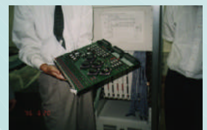
A processing board for UWBC (Ultra Wide Band Correlator)
