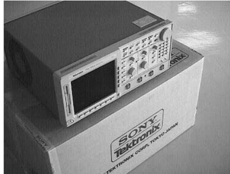
Figure 1. Giga-bit sampler, which is modified from Sony Tektronix TDS-784 series Digital Oscilloscope
