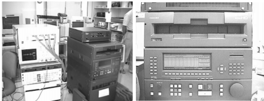
Figure 2. Giga-bit VLBI data recording system. Left picture shows observation system including sampler and interfaces. Right picture is the GBR-1000.
