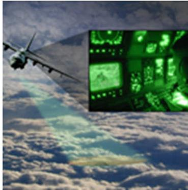
DARPA's Video Synthetic Aperture Radar (ViSAR) program seeks to develop and demonstrate an Extremely High Frequency (EHF) targeting sensor which operates through clouds as effectively as today's infrared (IR) sensors operate in clear weather.
