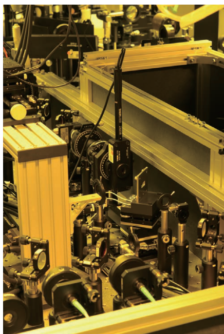
Figure 2 Measurement system for the electro-optic constant, r_{33} (transmission ellipsometric method without an aperture)
