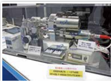
Compact, lightweight vacuum ion pump
