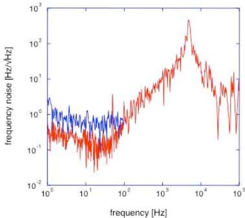
Fig.4 Frequency noise spectra of the I<sub>2</sub>-stabilized Yb:NPRO
