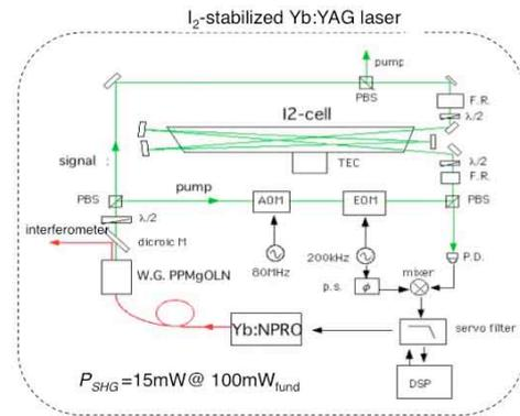
Fig.2 Schematic diagram of the  $I_2$ -stabilized Yb:YAG laser
