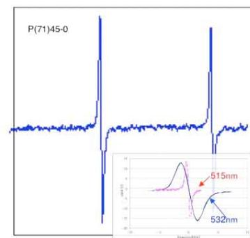
Fig.3 Saturated absorptin signal of  $I_2$  at 515nm
