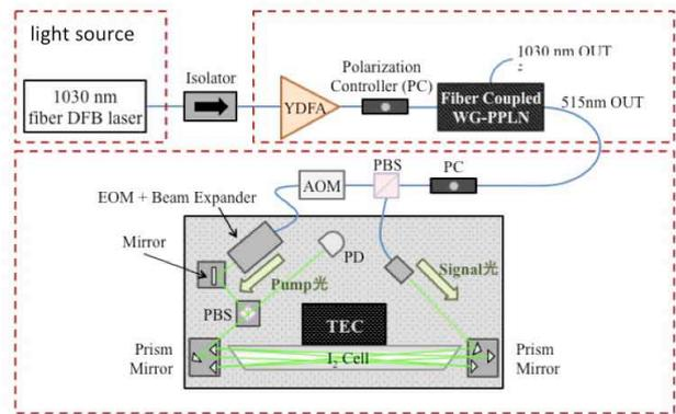
Fig.5 Configurations of breadboard model of I<sub>2</sub>-stabilized laser
