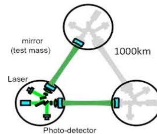
Fig.1 Configuration of the space gravitational wave detector DECIGO
