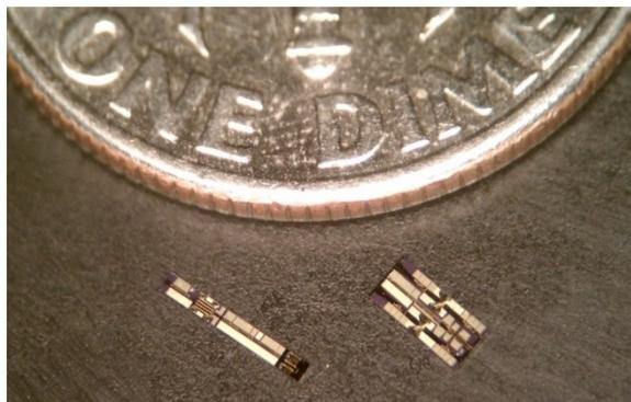
Figure 1: Monolithically integrated InP coherent receiver and transmitter photonic IC's.
