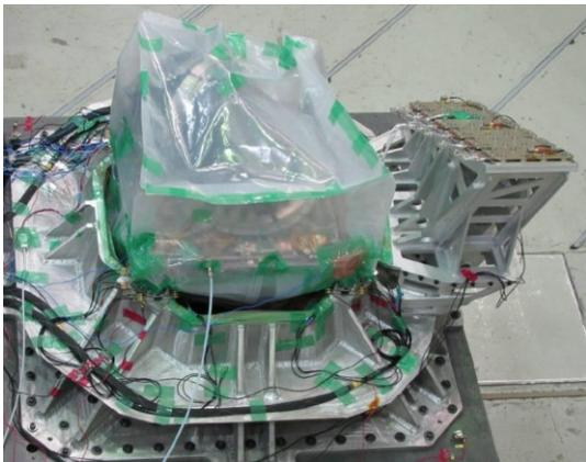
Figure 4. Alphasat LCT mounted on a vibration adapter, ready for vibration testing
