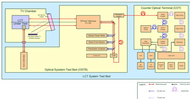
Figure 6. The optical system testbed for testing the Alphsat LCT (not all units of the generic OSTB shown are used)
