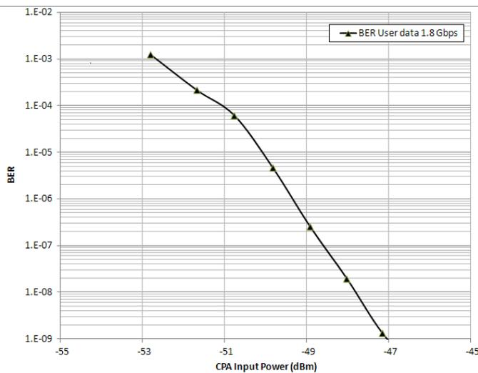
Figure 8. BER of LCT versus LCT CPA input power
