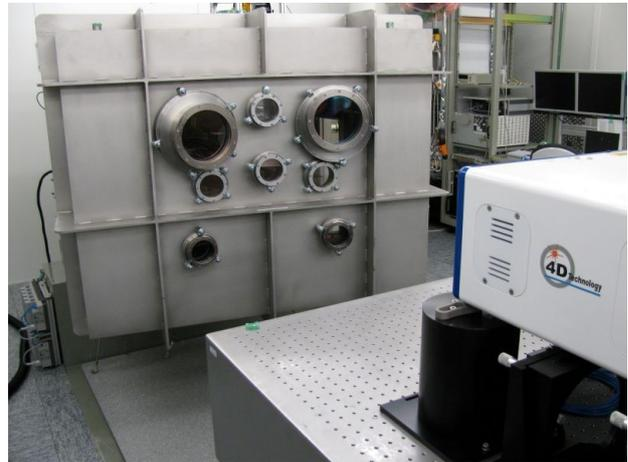
Figure 5. Thermal vacuum chamber for LCT performance verification with several optical windows for LCT access. The bigger windows allow access to the LCT CPA aperture to perform communication and wave front error measurements, while smaller windows allow access to the LCT pointing reference cube for pointing verification.
