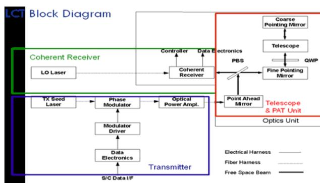
Figure 1. Tesat LCT block diagram.
