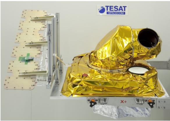
Figure 3. Alphasat LCT, equipped with MLI, with a Alphasat specific thermal Interface, mounted in its transportation frame
