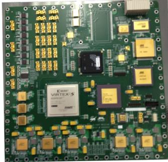
**Fig. 5.** Digital electronics board containing modems, processors, and memory, capable of supporting 10-Gb/s data rate. Developed based on flight-grade parts.
