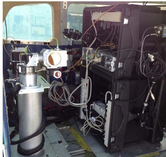
**Fig. 10.** Flight terminal together with electronics and laser integrated in a Cessna 206 aircraft.
