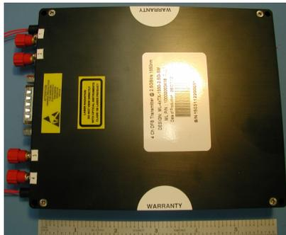
**Fig. 2.** The four-channel seed laser consisting of four DFB lasers, each modulated directly at 2.5 Gb/s.
