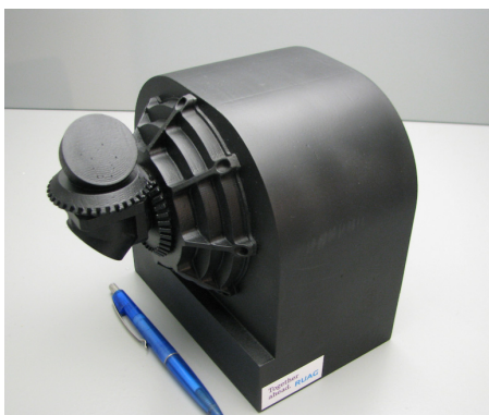
Figure 9 Optical Head Unit -Rapid Prototype, OPTEL-μ space terminal
