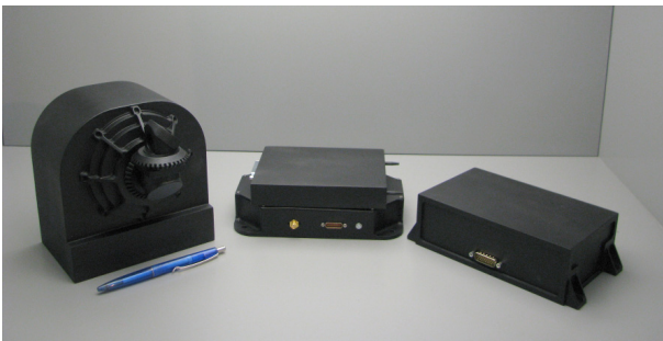
Figure 2 OPTEL \mu space terminal, 3 main units, rapid prototyping models (from left: Optical Head Unit, Laser Unit, Electronics Unit)
