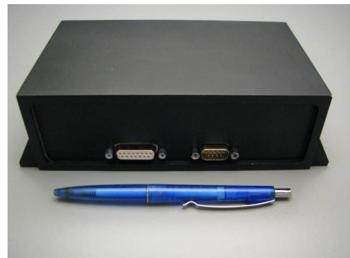
Figure 10 Electronics Unit -Rapid Prototype, OPTEL-μ space terminal
