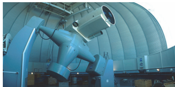
Figure 9. The telescope of ESA's optical ground station (OGS) on Tenerife used for the experiments is a Zeiss 1 meter Ritchey-Chrétien/Coudé telescope supported by an English mount.
