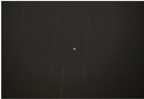
Figure 3. Image of ARTEMIS and star tracks during of pointing
