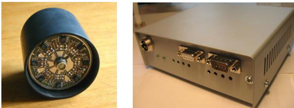
Figure 11. Multi-element photodetector, QPD module and Electronic module
