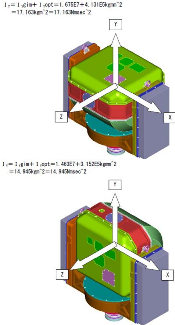
Fig. 10 Typical inertia condition around the azimuth axis.
