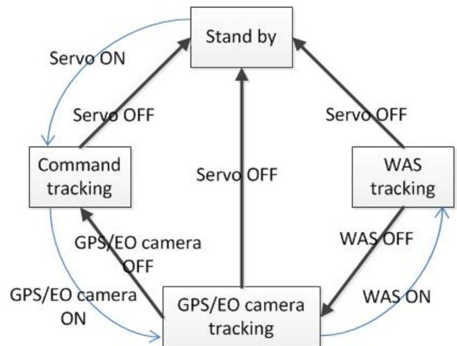
Fig. 12 Upper level control scheme for the gimbals.
