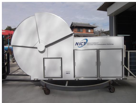
Fig. 1. Overview of the compact ground station.
