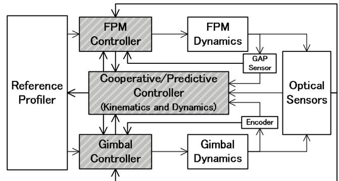
Fig. 11 Lower level control scheme.
