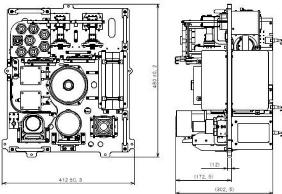
Fig. 7 Size of the optical module.
