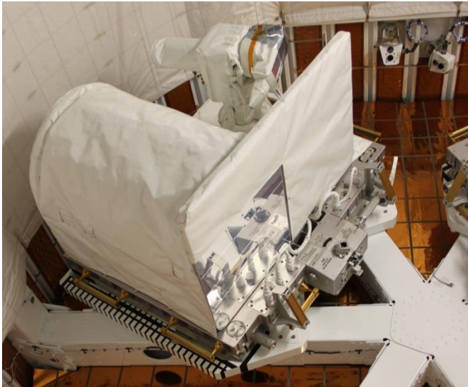
Fig. 1. OPALS payload in flight configuration during integration with the launch vehicle. The two-axis gimbal-mounted optical transceiver (shown here with a protective cover on) and the barrel-shaped seal container give OPALS its distinctive look.
