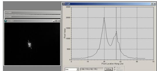
Figure 15. Image art 3307. Line slice of laser beacon beam via clouds
