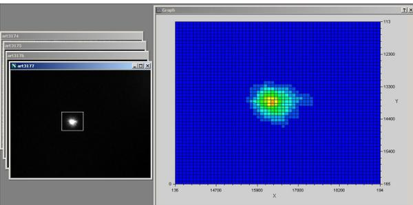
Figure 6. Image art 3177. 3D view of laser beacon from ARTEMIS via clouds
