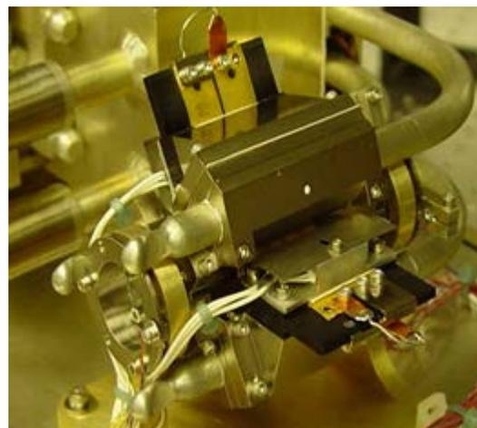
Figure 2: Most recent version of laser head. Six LDAs produced 3.6 J of pump energy. Cooling is completely conductive with no water channels.
