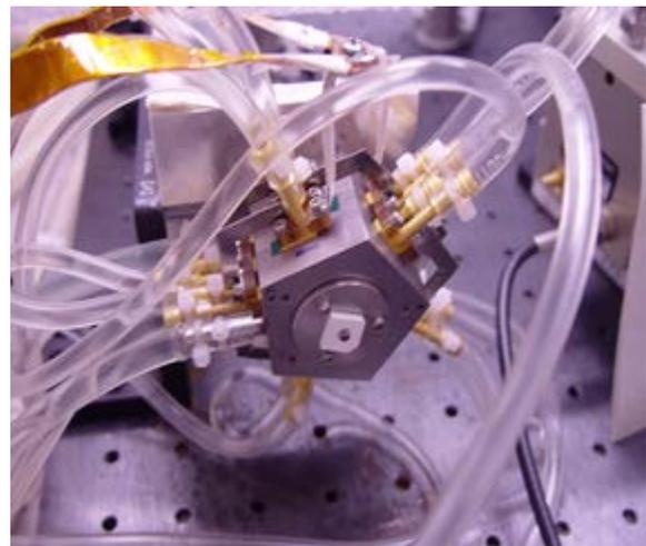
Figure 1: Early version of laser head containing laser rod and pump LDAs. Ten LDAs produced 3.6 J of pump energy. There were 22 water channels
