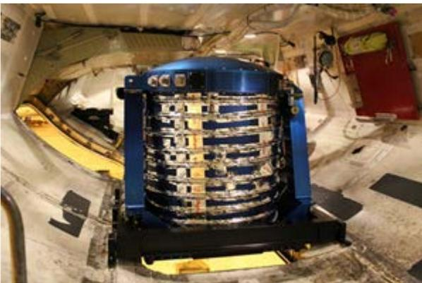
Figure 4: Compact-packaged coherent lidar optics in the cargo level of the NASA DC-8. The optics canister comprises the lidar transceiver, a beam-expanding telescope, an optical wedge for beam scanning, and a pressure window.
