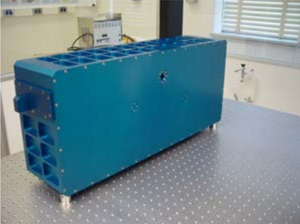
Figure 3: First version of a compact-packaged, coherent lidar transceiver. The transceiver comprises the pulsed 0.25-J, 10-Hz laser, CW seed laser, lidar transmit-receive switch, and dual-balanced detectors. The beam exits from the side hole.
