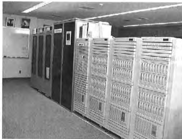
Photo. 4 KSP type correlator for 3 stations and 3 baselines
