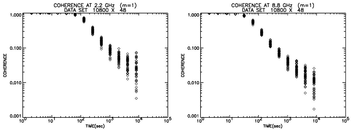
Figure 5. Coherence calculated using residual phase data after a linear drift is removed versus integration time for 2.2 GHz (left panel) and 8.8 GHz (right panel).
