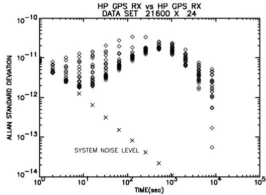
Figure 3. Root Allan variance calculated for 24 sets of phase data. Each data set spans 6 hours. Measuring system noise level is represented by symbol "X".
