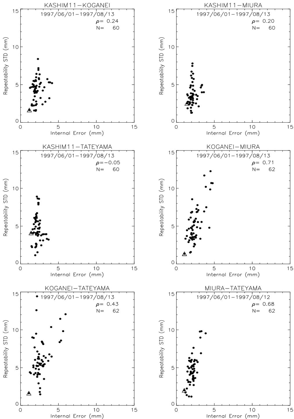
Figure 2. Repeatabilities and formal errors by baseline for the period between June 1, 1997 to August 13, 1997. Open triangles represent data for 120-hour observations.  $\rho$  is a correlation coefficients between parameters.
