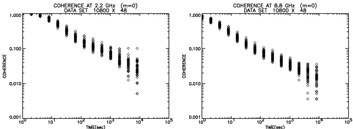
Figure 4. Coherence calculated from the phase data versus integration time for 2.2 GHz (left panel) and 8.8 GHz (right panel).
