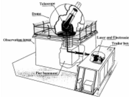
Keystone SLR view including dome building and trailer box housing laser and electronics
