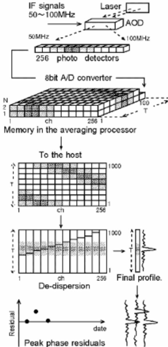
Figure 2. Data flow from the AOS to the host computer.
