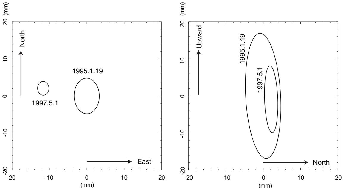
Figure 1. Comparison of KASHIM11 position estimated from two joint experiments. The ellipses express one sigma uncertainties of the estimated position (a) in the horizontal plane and (b) in the vertical plane.
