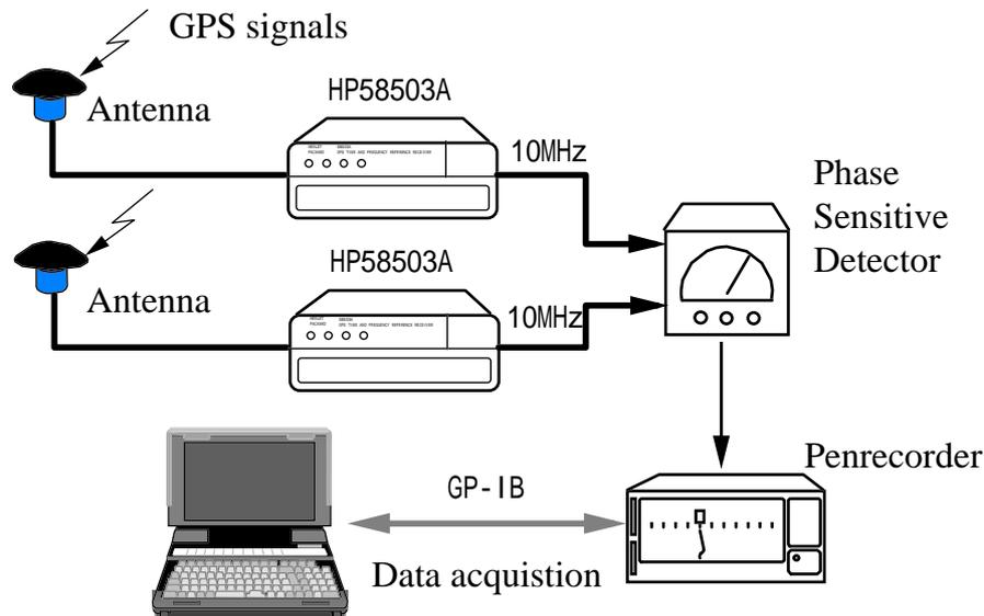
Figure 1. Schematic block diagram of observation system.
