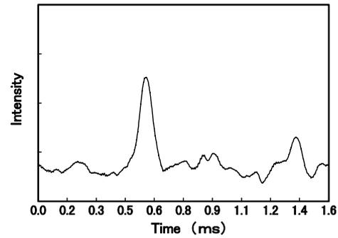
Figure 3. Pulse profile for PSR1937+21 at 2GHz band. Integration time is about 14 minutes and receiving bandwidth is 150MHz.
