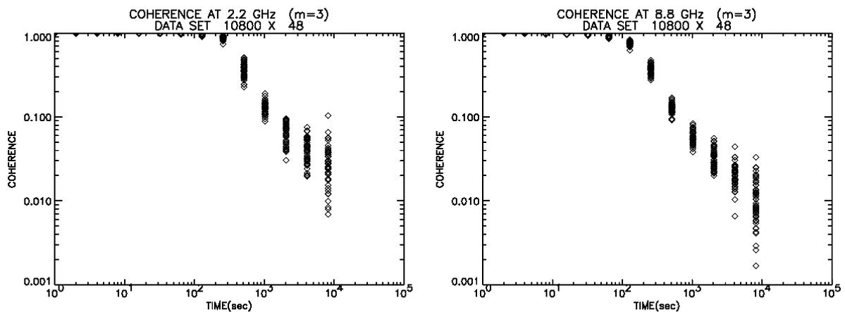
Figure 6. Coherence calculated using residual phase data after a third order polynomial fit versus integration time for 2.2 GHz (left panel) and 8.8 GHz (right panel).
