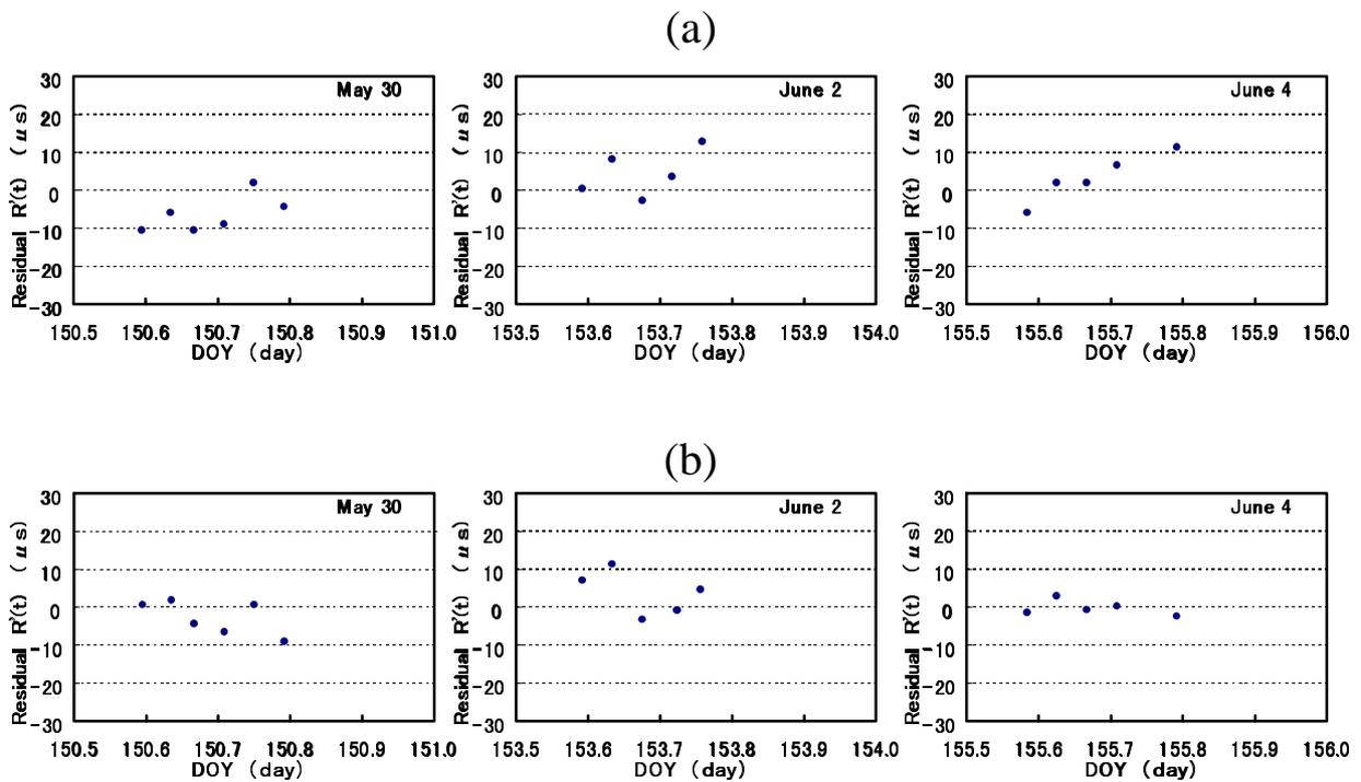
Figure 4. Residuals of peak phase for PSR1937+21. (a) Observation data using a database calculated by VAX TEMPO. (b) The same days' data corrected by a database calculated by UNIX TEMPO.
