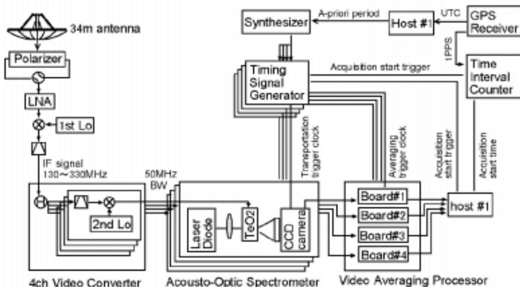
Figure 1. Block diagram of millisecond pulsar observation system at CRL.
