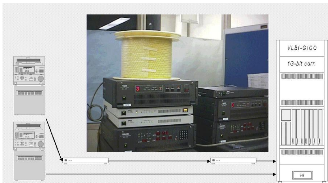
Figure 4. Giga-bit optical transmitter SPO1152TX/RX test in VLBI correlation.
