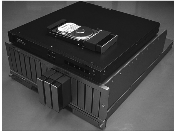
Figure 1. There are a removal disk unit which has the hot-plug function, previously described ADS1000, the disk array with fourteen independent 400GB serial ATA drives and 1U PC server equipped VSI2000-DIM board.
