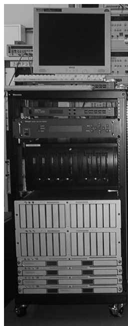
Figure 2. The cluster PCs and disk arrays are set up on the lower half of the rack.
