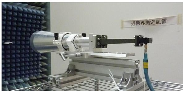
Figure 3. Testing IGUANA daughter feed at MET-LAB in Kyoto UNIV. Physical dimensions are  $\phi 133\text{mm}$  (No.1),  $\phi 120\text{mm}$  (No.2)  $\times L300\text{mm}$
