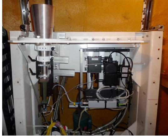
Figure 1. Prototype of Iguana Feed install at Kashima 34m antenna. SEFD is 1000 – 1500 Jy in 6.5–14 GHz frequency range.
