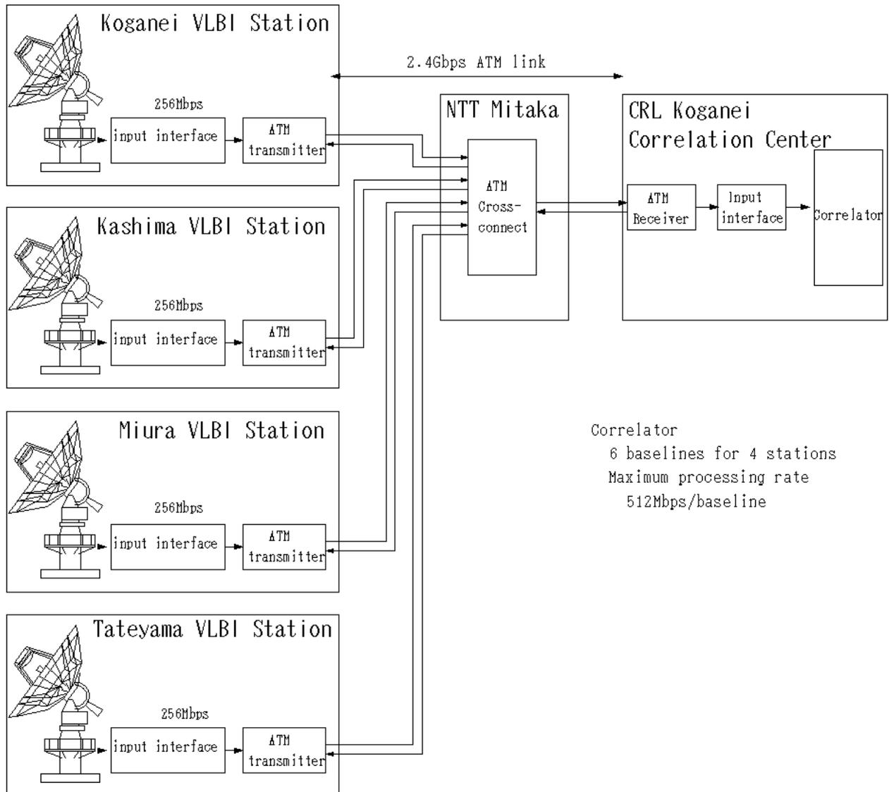
Figure 1. Block diagram of the realtime VLBI in KSP project.
