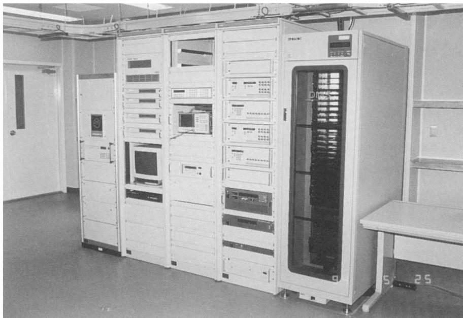
*KSP/VLBI system at Koganei station. From left: Weather station, antenna front-end control, calibration system, backend terminal, and automatic tape loading unit(DMS24).*
