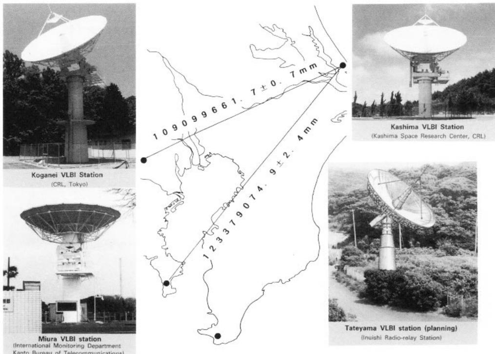
Figure 1. Configuration of KSP and the baseline length.
