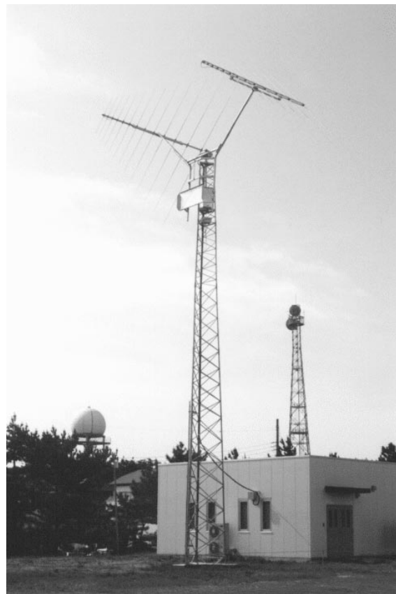
Figure 1. Antenna for detection of decametric radio waves at Kashima.
