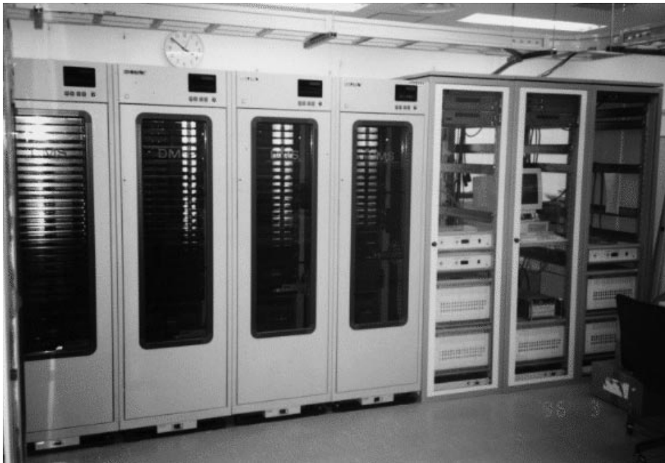
Figure 4. Developed multi-baseline correlation processing system. From left : 4 DMS (Digital Mass- storage System: automatic tape changer)
