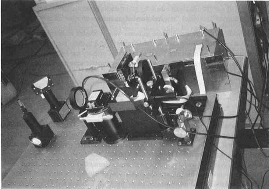
Fig. 15 An acousto-optical spectrometer (AOS) developed at NRO. An optical diode-laser is used. The frequency resolution and the band width are 40 kHz and 40 MHz, respectively.
