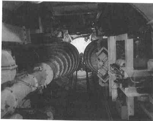
Fig. 8 Feed cone internals. Feed horns and receivers are attached to rails and move up to the cassegrain focus from the coontrol room.
