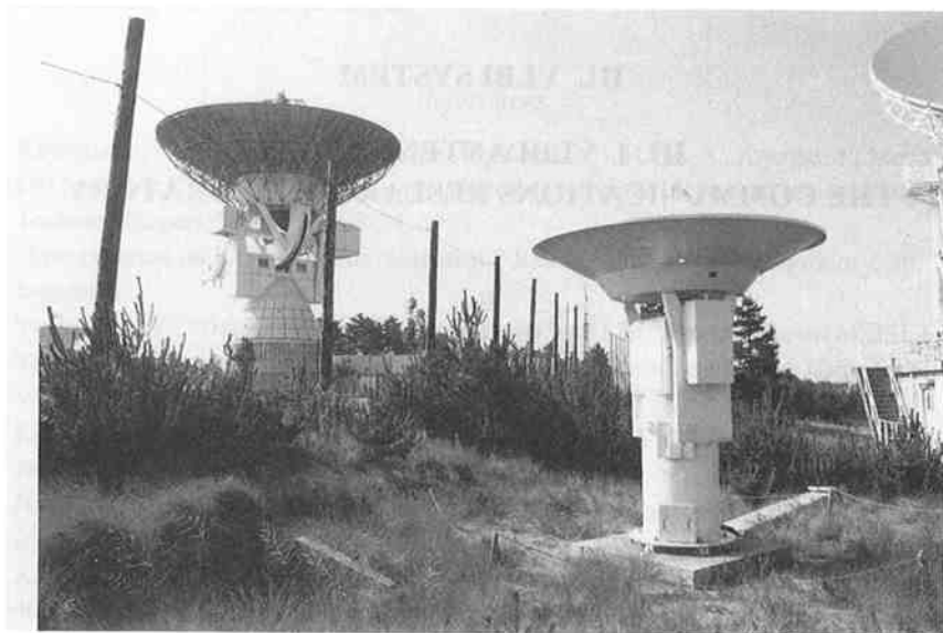
Fig. 1 26-m antenna (left) of the Kashima Space Research Center and 3-m antenna (a mobile station).
