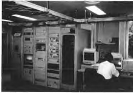
Fig. 8 VLBI data acquisition system at Koganei (The systems used at all four sites are identical)
