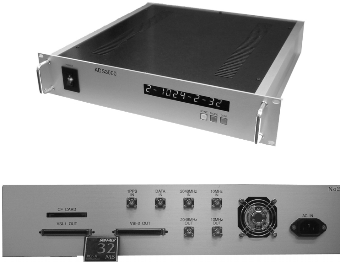
FIG. 2.—Front and rear view of the ADS-3000. FPGA logic is easily programmable with a CompactFlash card. A 2048 MHz PLL-output port and 2048 MHz input port are directly connected in most cases. A 2048 MHz reference signal can be distributed to other units using these ports. [See the electronic edition of the PASP for a color version of this figure.]
