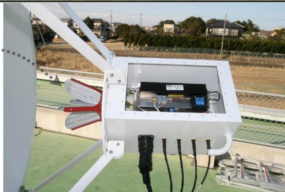
Dual-Polarized Quad-Ridge Horn Antenna (2-18 GHz)
