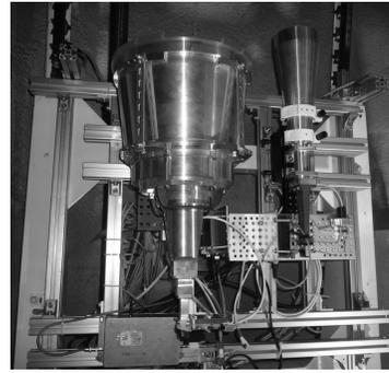
**Fig. 2** Picture of broadband feed system of Kashima 34m antenna. NINJA feed in the left side and IGUNA-H feed in the right hand side.
