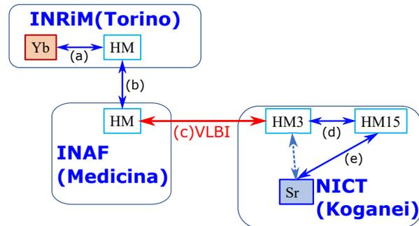
**Fig. 2** Block diagram of the frequency chain between INRiM and NICT. Since optical lattice clocks (Yb,Sr) are operated intermittently with several hours of run, hydrogen masers (HM) are used as a flywheel to keep the frequency and link the frequency chain. Frequency ratio between each pair of nodes are measured, and the longest link was made by the VLBI observation.
