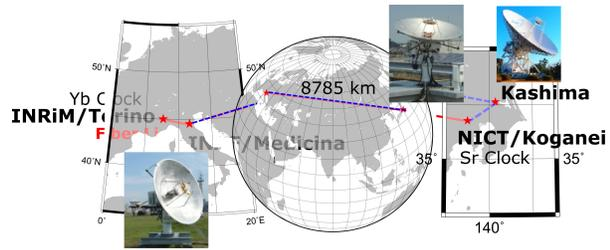
**Fig. 1** Overview of the frequency link experiment between Italy and Japan. Reference frequency of Ytterbium lattice clocks operated at INRiM was provided to Medicina (INAF) by fiber link. Frequency link from Medicina to Koganei (NICT) was made by using VLBI observation. Kashima 34-m antenna participated the VLBI experiment to enable VLBI between 2.4 m antenna pair via NHS VLBI scheme.
