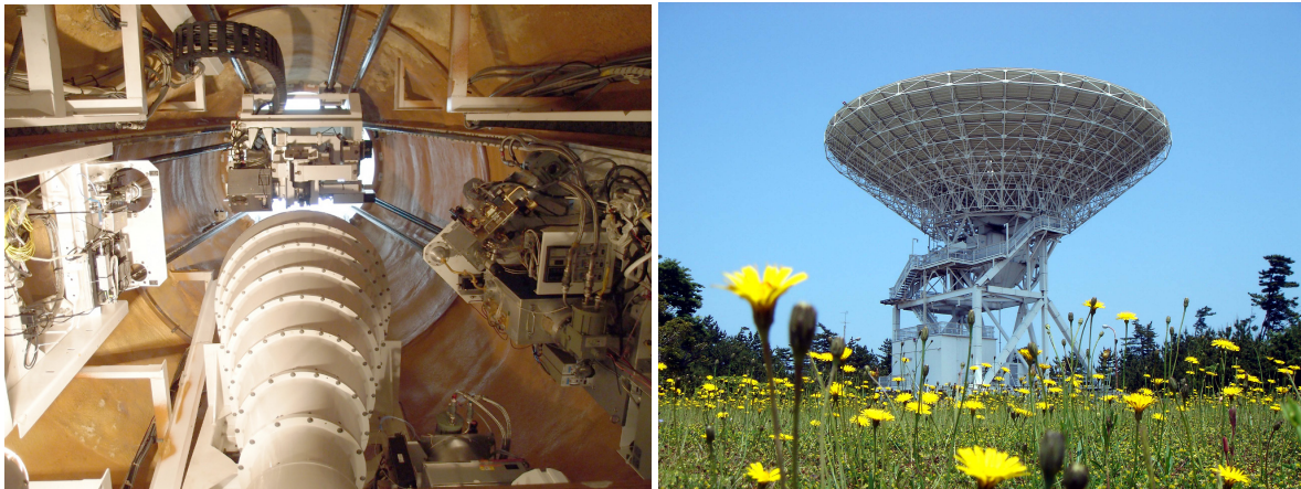
Fig. 3 Left: Bottom view of the Kashima 34-m antenna receiver room. Receivers are separated into four groups and mounted on one of four trolleys. Observing receiver is changed by exchanging the trolleys at the focal point (center). Right: Kashima 34-m antenna and flowers.
