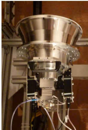
Fig. 2 Broadband ‘NINJA’ feed mounted on Kashima 34-m antenna.
