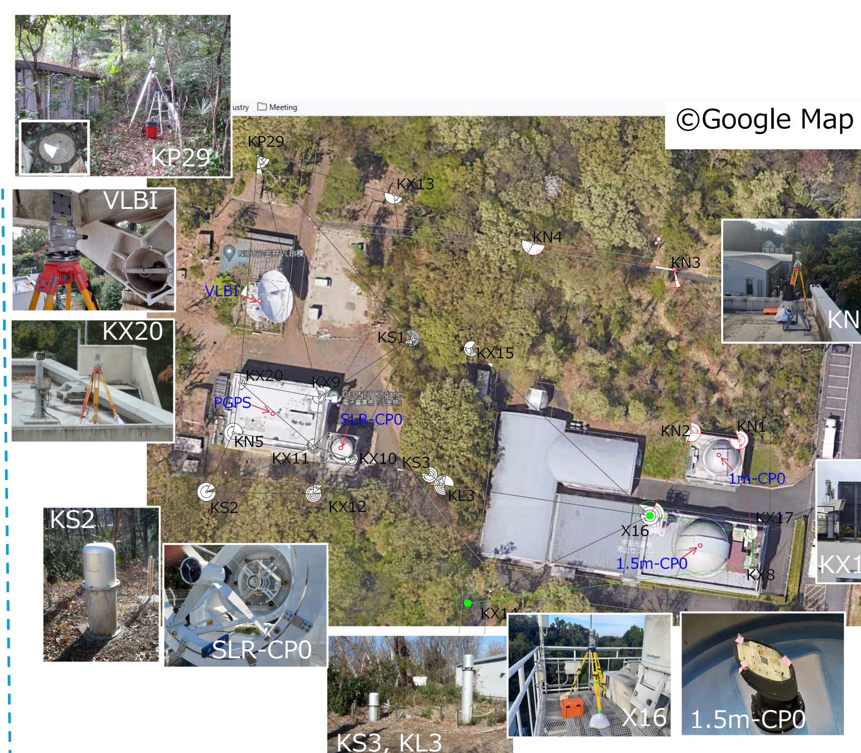
Fig.5 Site view of Koganei site and ground marker/monuments used for local tie survey.
