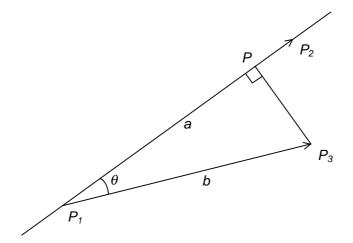
Suppose the coordinates of points  $P_1$ ,  $P_2$  and  $P_3$  are being measured. When a line perpendicular to the straight line between  $P_1$  and  $P_2$  is drawn from point  $P_3$ , the range  $(\overline{P_1 P})$  between  $P_1$  and  $P_2$  can be measured.
